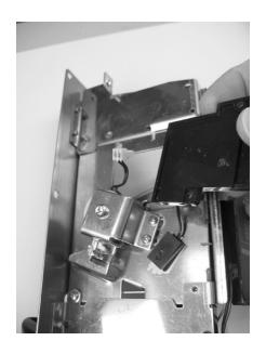
8) When complete, position the round opening in the fixed side sensor over the ramp screw that protrudes and push the fixed sensor assembly in loosely.
