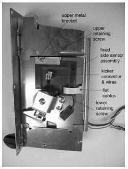
It is extremely important that the flat cables and kicker wires are not folded, kinked or stressed in any way. In addition be extremely careful that the the flat cable does not rub against any surface that would either scratch or cut into the cable. Damage to the flat cables or kicker wires is not covered under warranty and can only be repaired at the factory.
