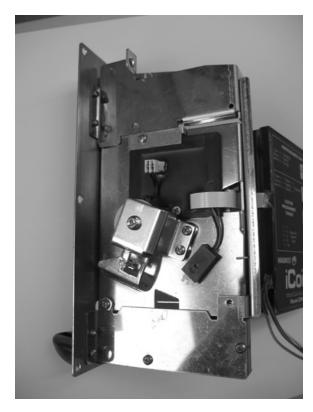
4) Remove kicker connector by gently pressing down to release locking mechanism on connector.
