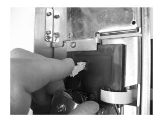
5) Use the philips screwdriver to remove upper retaining screw and upper metal bracket on the fixed side sensor assembly.
