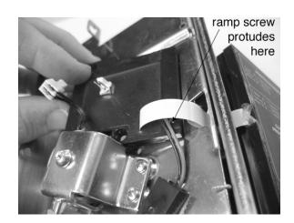
9) Turn the coin acceptor over. If necessary gently lift the door side sensor assembly to the left. You may now clean the inside of the acceptor, including the face of the door side sensor assembly in the same manner and with the same precautions as stated previously.
