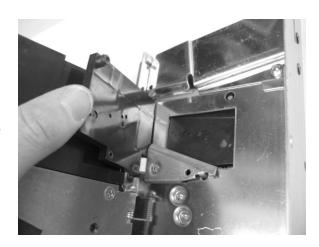
10) Once complete, place the door side sensor assembly in position by locating the upper right post in the hole in the metal side. Ensure that the flat cable attached to the bottom of the door side sensor assembly is positioned correctly.
