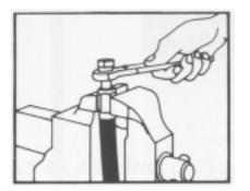
Place a generous amount of grease on insert portion of reuseable end and on the inside of the hose. Screw insert fully into shell until the hex portion of the insert is in full contact with the shell.
