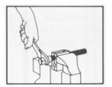
Clamp hose lightly in vise. If desired oil outside of hose. Turn shell portion of reuseable end on to hose until it bottoms onto hose. Back off shell one full turn or approximately 1/4".
