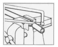
Cut hose square to the desired length using a cut-off wheel or a fine-toothed saw. Clean the end of the hose from any debris.
